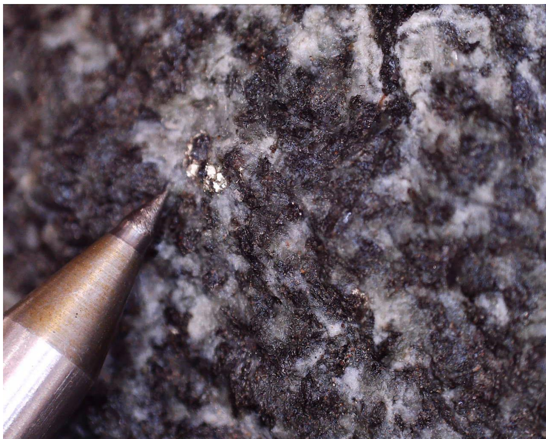
Figure 13. Coarse-grained pyrite in coarse-grained gabbro in centre of sill.
