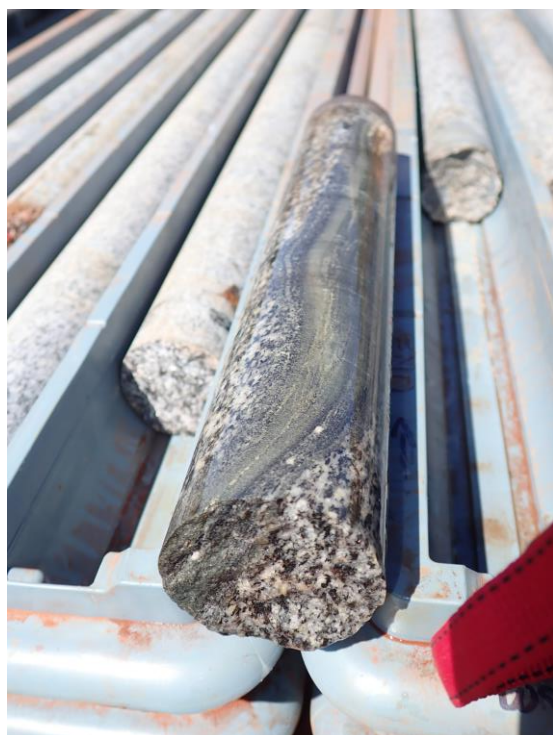
Figure 4. Chalcophyrite “seam” and iron oxide “raft” within narrow shear in biotite granodiorite (WSDD002 – 231.6m).
