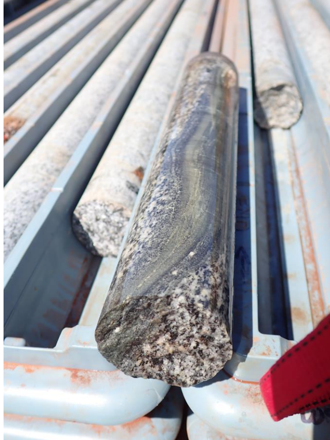
Figure 2. Chalcopyrite “seam” in shear zone within biotite granodiorite (WSDD002 – 231.6m).
