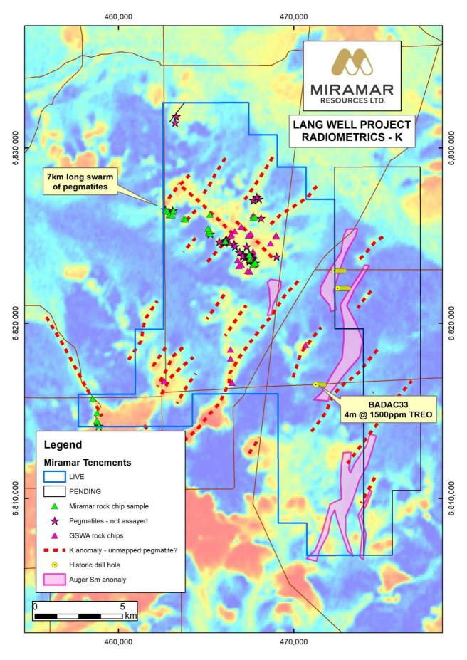
Figure 4. Lang Well Project showing K anomalism and auger Sm anomalies.
