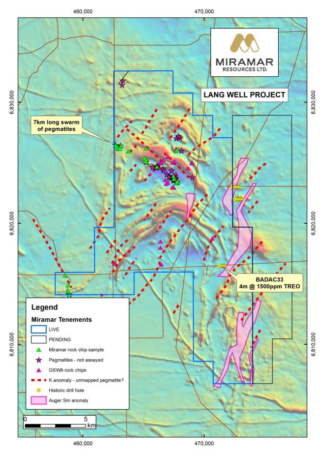
Figure 1. Lang Well Project pegmatite occurrences and Sm anomalies over magnetic image.
