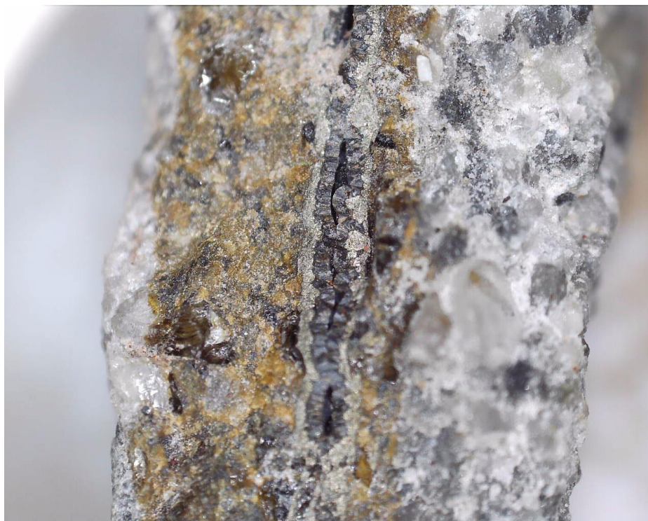
Figure 3. GJAC714 (58-59m EOH) showing quartz vein and sulphides in a porphyritic unit.
