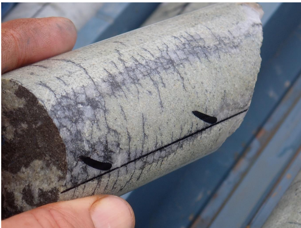
Figure 4. Thin low-angle quartz-sulphide veinlet in GJDD002 with specks of visible gold.
