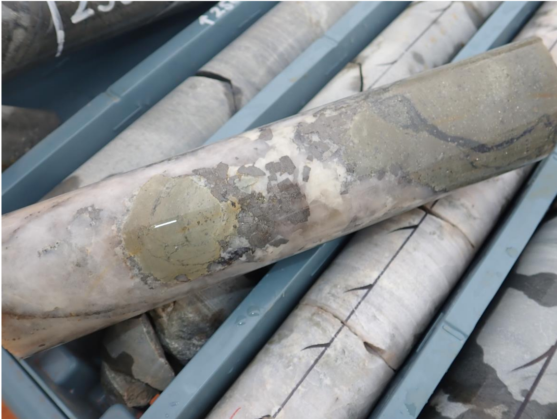
Figure 4. Quartz/sulphide breccia with coarse grained arsenopyrite (GJDD002).
