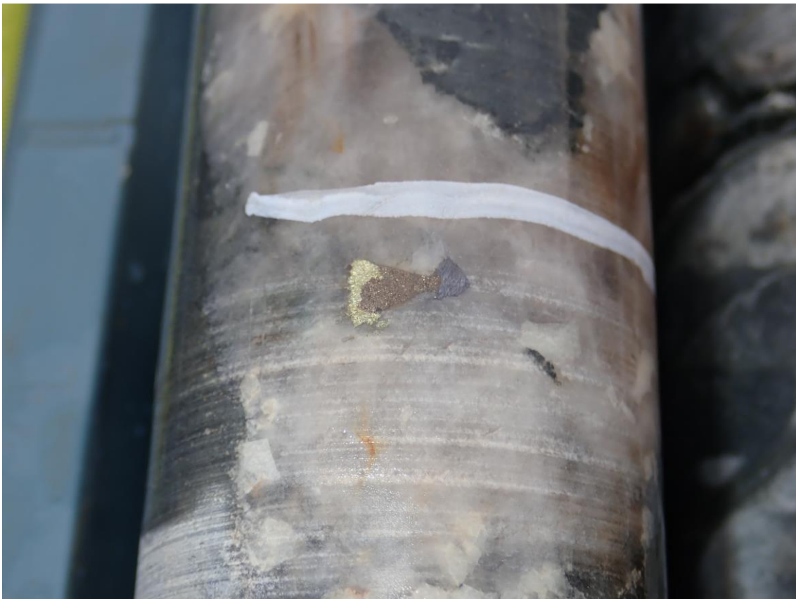
Figure 5. Quartz/sulphide breccia showing chalcopyrite, pyrrhotite and galena (GJDD002).
