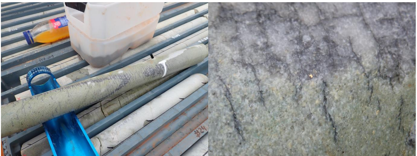
Figure 3. Quartz/sulphide vein with visible gold in altered hanging wall sandstone (GJDD002 – 124.7m).
